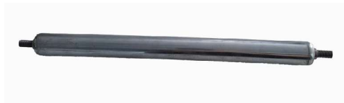
Steel roller for conveyor systems with a diameter of 25 mm, M8 thread, and a length of 600 mm. Made of galvanized steel.
