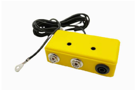
Grounding box with safety resistors for use as part of the main grounding measure Wrist strap for employees Design / Construction: 2 x 10 mm push button, 1 x 4 mm banana plug to 4 mm ring lug
